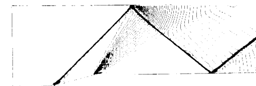
Fig. 9 Adaptive grid solution, pressure contours ( \Delta p=0.05 )
