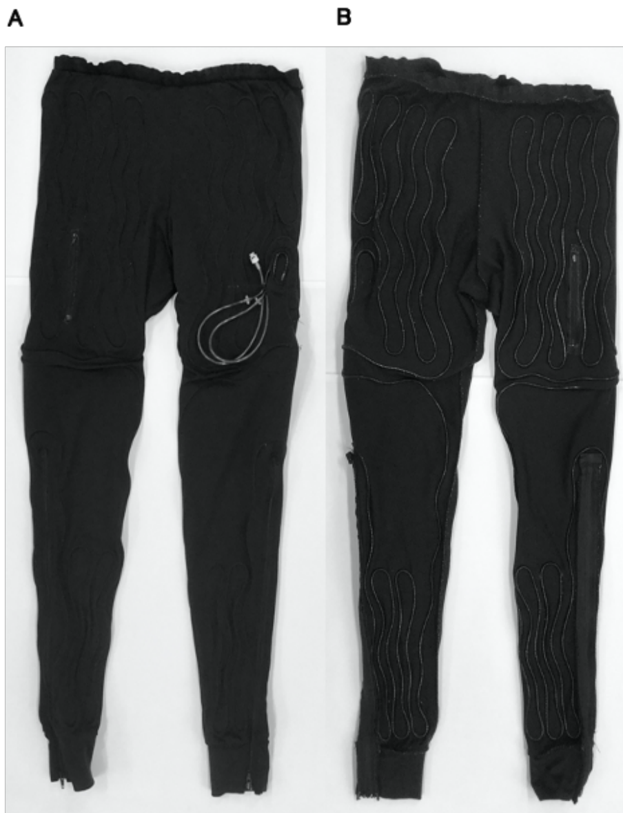
Figure 2-1. The water perfusion trousers used in this experiment. A and B show and outside and inside view of the trousers, respectively.
