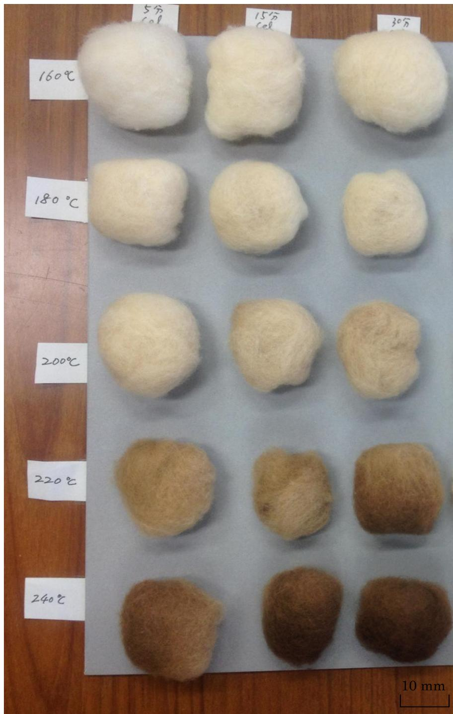
Fig.2-12 Cotton fiber after heating
