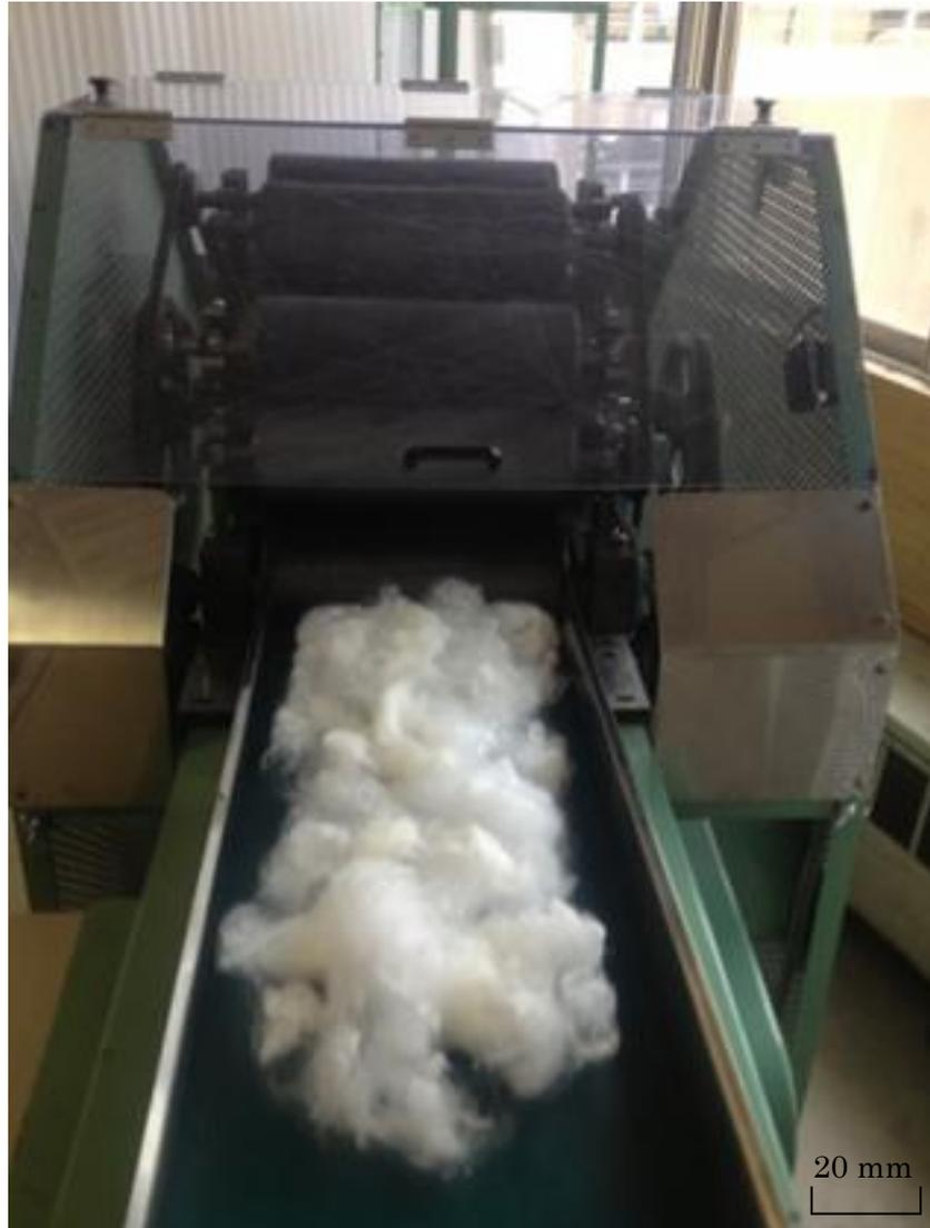
Fig.4-2 Carding machine with cotton/PP mixture fiber
