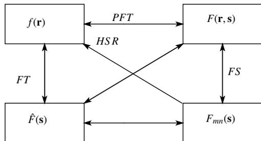
**Fig. 3** Periodic Fourier transform (PFT), harmonic series representation (HSR) and Fourier transform (FT).  $\hat{F}(\mathbf{s})$  is the Fourier spectrum,  $F(\mathbf{r}, \mathbf{s})$  is the  $s$ -periodic spectrum, and  $F_{mn}(\mathbf{s})$  is the harmonic spectrum.
