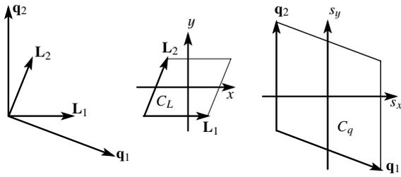
**Fig. 2**  $\mathbf{L}_1$  and  $\mathbf{L}_2$  are basic vectors.  $\mathbf{q}_1$  and  $\mathbf{q}_2$  are Bragg basic vectors with  $\mathbf{L}_i \cdot \mathbf{q}_j = 2\pi\delta_{i,j}$ .  $C_L$  and  $C_q$  are the  $\mathbf{r}$  unit cell and the  $\mathbf{s}$  unit cell, respectively.
