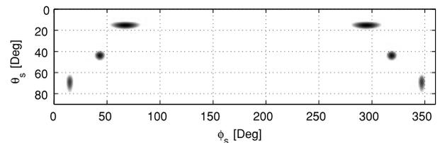
**Fig. 5** Scattering cross section  $\sigma(\theta_s, \phi_s | \theta_i, \phi_i)$  by the first order solution. Gray scale image. There are 6 black footprints representing the main-lobes of diffraction beams.  $\theta_i = \pi/6$ ,  $\phi_i = \pi$ ,  $\sigma_h = 0.1\lambda$ , and  $\kappa = 5\lambda$ .
