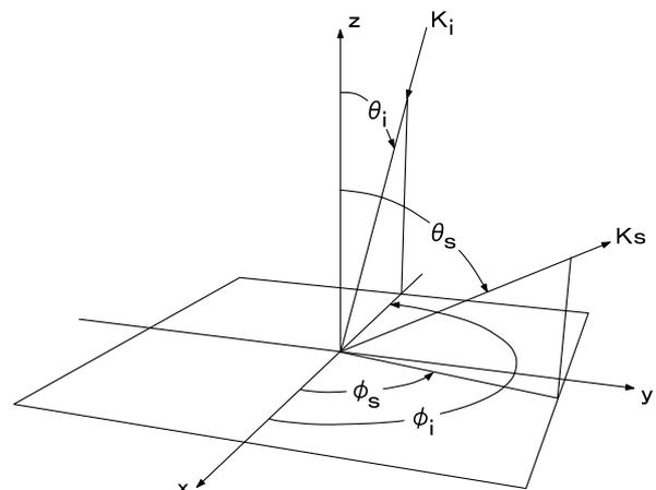
Fig. 4 Scattering of a plane wave.  $\mathbf{K}_i$  is the incident wave vector and  $\mathbf{K}_s$  is a scattering wave vector.
