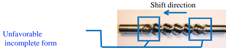
Fig.1・16 Work piece shift during a rolling process
