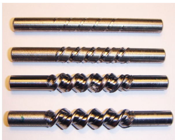
Fig.5・12 Photographs of \phi 5.9\text{mm} work piece at every penetration stage
