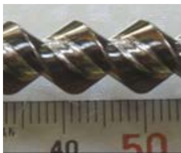
Fig.3.1 An example of form rolled gears ( m_n = 1.25 , z = 2 , \beta = 45^\circ )
