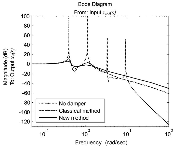
**Fig. 4.5. Gain of frequency response of  $x_4(s)/x_{tr2}(s)$**
