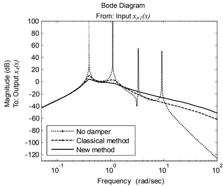
**Fig. 4.4. Gain of frequency response of  $x_4(s)/x_{tr1}(s)$**
