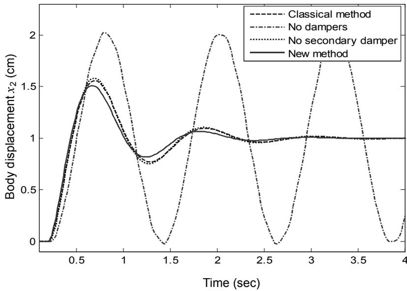
**Fig. 3.2. Unit-step response of train**
