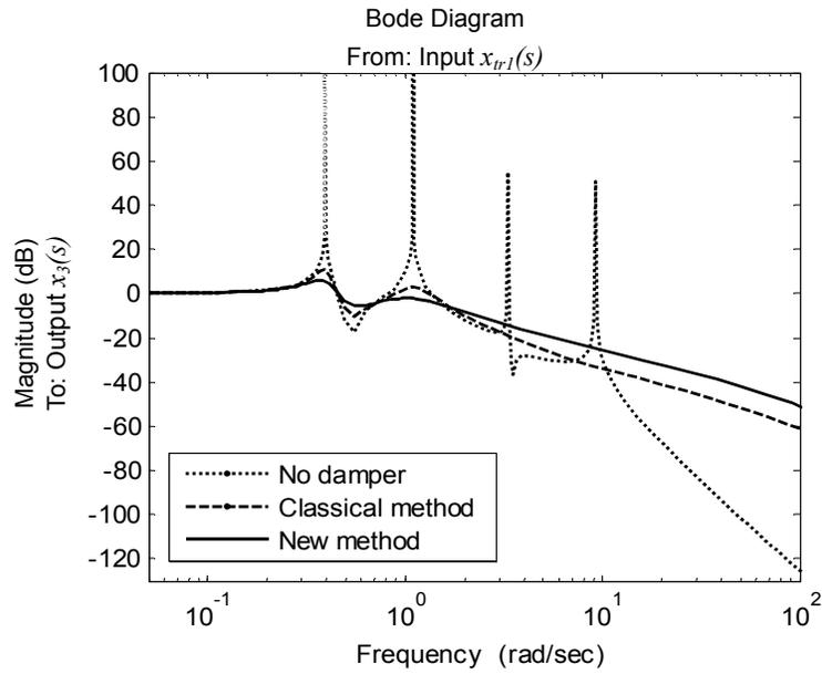
**Fig. 4.2. Gain of frequency response of  $x_3(s)/x_{ir1}(s)$**
