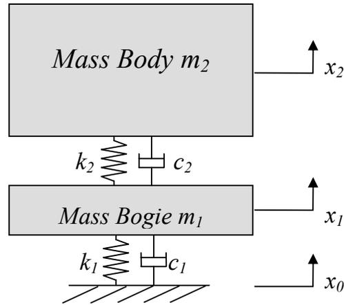
**Fig. 2.1. Two-DOF suspension system model**
