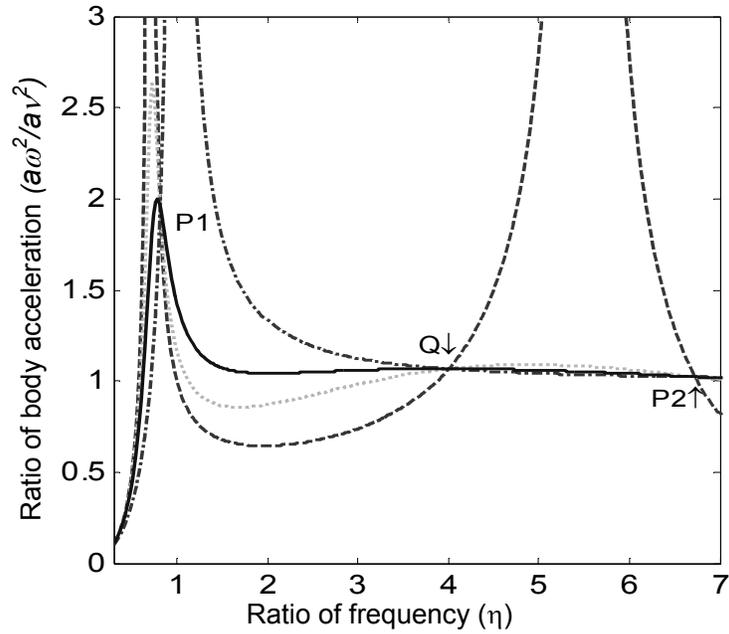
Fig. 2.3. Three fixed points in frequency response curves
