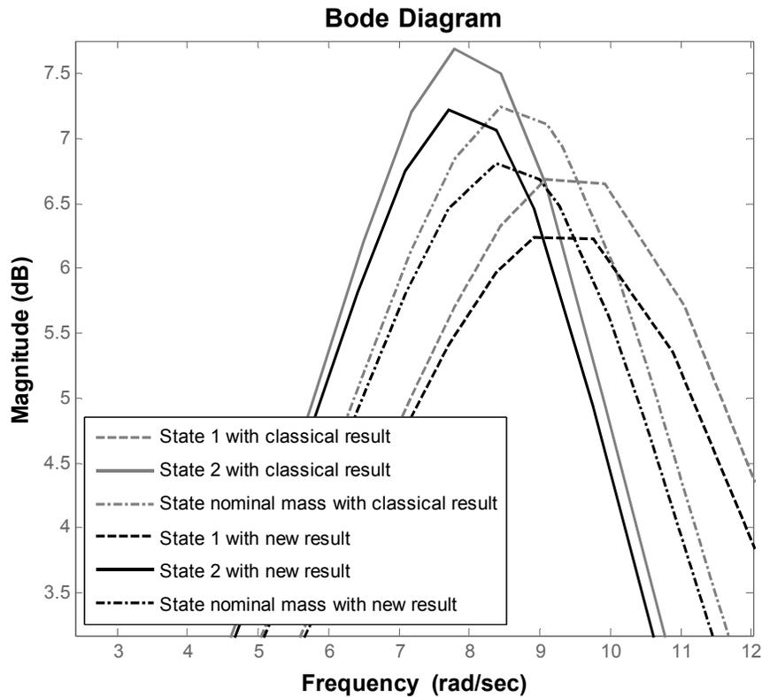
**Fig. 5.4. Close up of frequency responses by change in mass**
