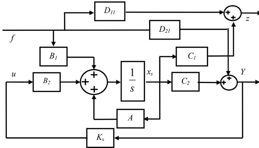
Fig. 2.5. Block diagram of feedback control system
