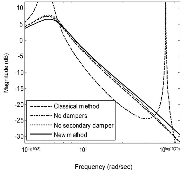
**Fig. 3.1. Frequency responses of suspension system**
