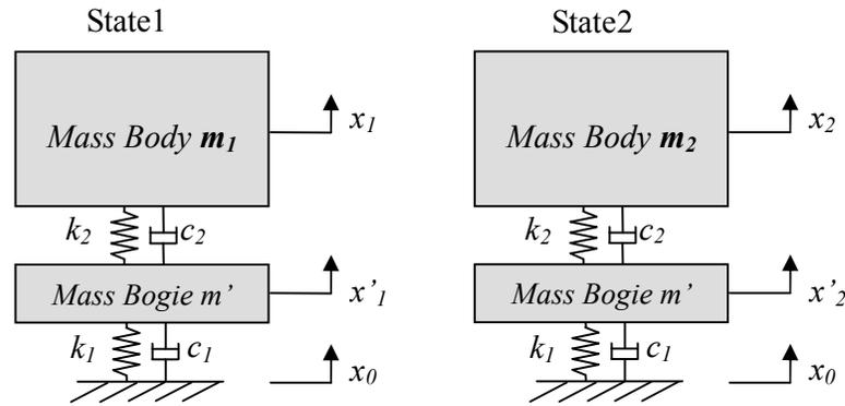
**Fig. 5.1. Two states of mass of proposed system**
