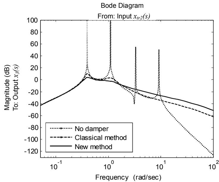
**Fig. 4.3. Gain of frequency response of  $x_3(s)/x_{ir2}(s)$**
