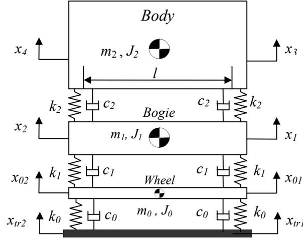
**Fig. 4.1. Six-DOF suspension system model of train**
